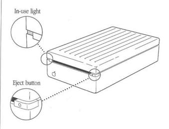
As a last resort, if you cannot eject a disk any other way, insert a straightened-out paper clip or similar object into the access hole to the right of the disk slot. Push carefully on the paper clip until the mechanism releases the disk. Do not force the mechanism by pushing too hard.
