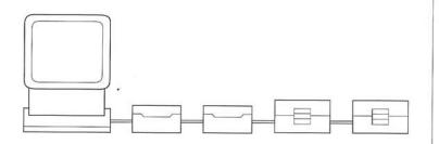
Up to four devices can be connected to your Apple II in a daisy chain. Your SuperDrive or SuperDrives should be nearest to the computer. To connect another drive to your SuperDrive, follow these steps:
