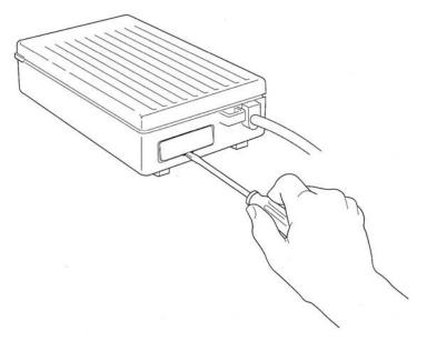
3. Plug the second drive's cable into the connector on the back of the first drive and tighten the retaining screws.
