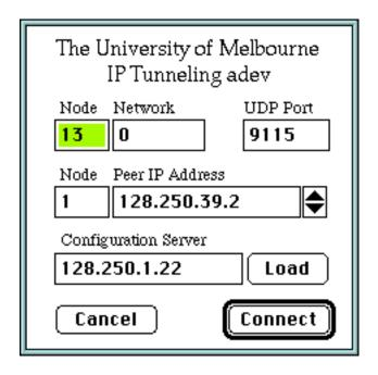
The **Node** field is the AppleTalk node number for this Macintosh. Node numbers are chosen (at random) by the UAR or AppleTalk network administrator and are uniquely assigned to the IP addresses of Macintoshes running *IPTnnl* or UAR "tnnl" interfaces. Valid node numbers lie in the range 1 - 253.
